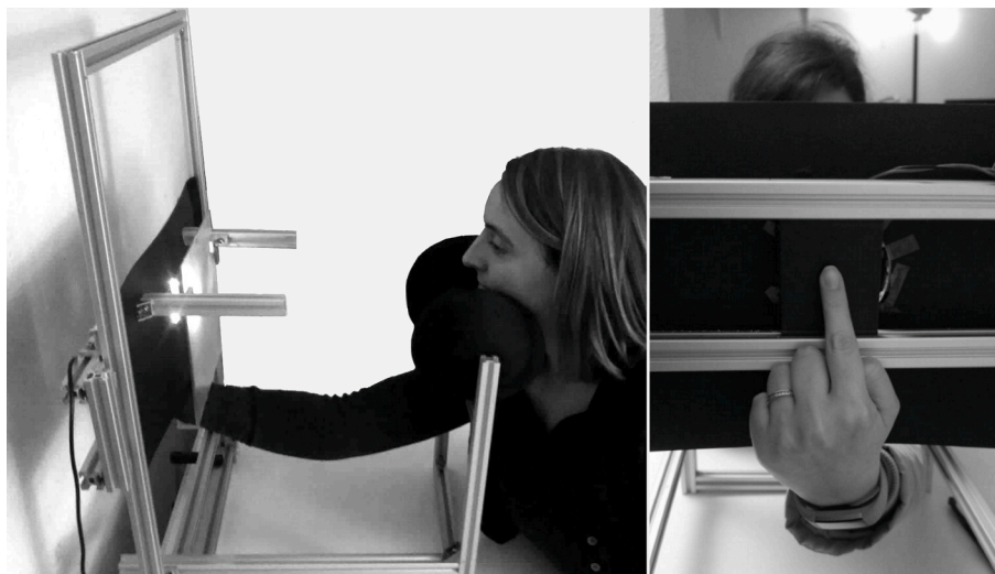
Fig. 1. Experimental setup. The left panel shows a participant reaching for the stimuli in the bimodal condition. The right panel shows a detail from the back side. Note that LED lights surrounded the aperture behind the black panel to control lighting conditions.
