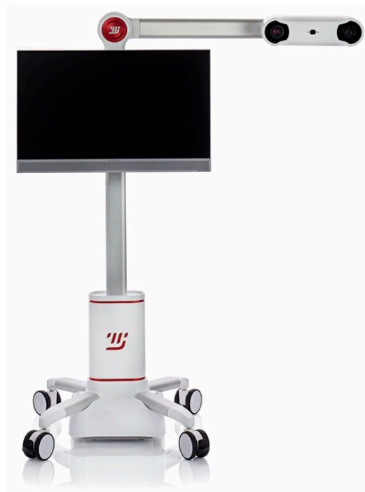
Figure 1. The ModJaw device with a camera based on 3D stereophotogrammetry to record mandibular movements on STL models.
