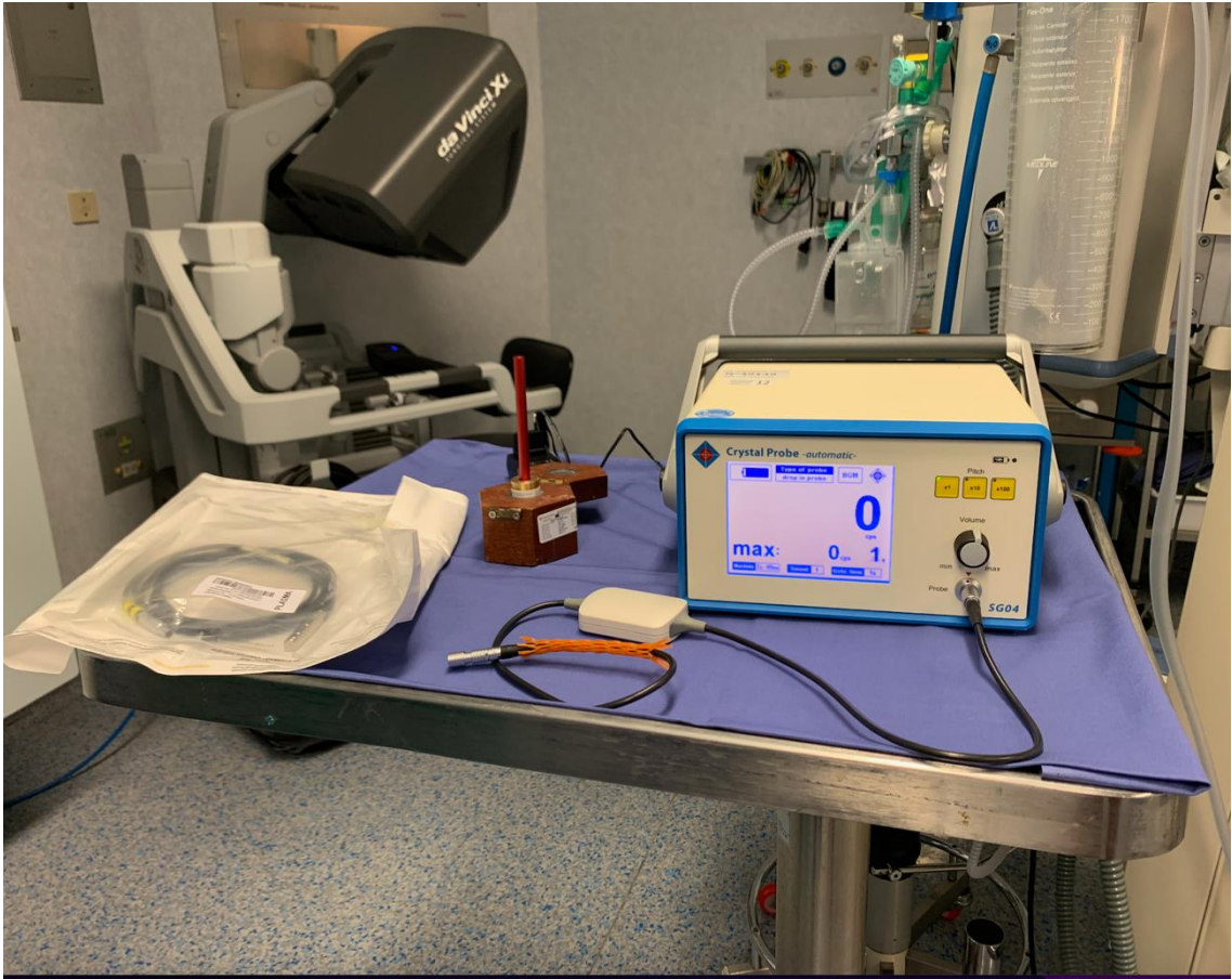
Figure 14. Standard set-up of the Crystal Probe within the operating room. The flexible cable is sterilized after each utilization (on the left), while the connecting cable to the main case is reused and stored (on the right).
