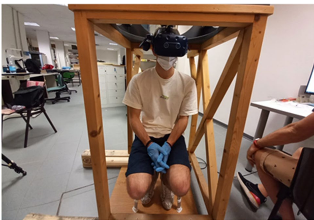
Fig. 2 The experimental setup. Thanks to a top-down forehead support, the wooden structure ensured a good head restraint while at the same time leaving free space for arm/hand movements in front of the participant
