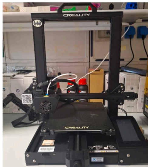
Figure 51. Creality 3D printer. Extrusion based 3D printer.
