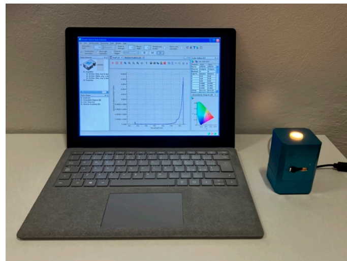
Figure 2. Representation of the spectrophotometer used for the detection of the color of the materials tested in the different laboratory conditions. CIELAB data were collected.
